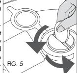
repeat at least once, then screw up the cap firmly with a coin and replace the rubber bung (15).
