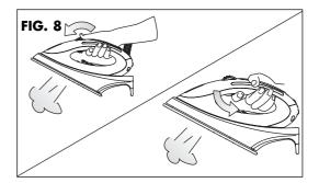
To obtain **continuous steam** rotate the wheel forwards until it locks into place.
