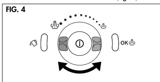
NB: When you turn the iron on, you are recommended to turn the regulator to the maximum steam position.
