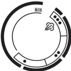
**Remember that the steam function can only be used when the thermostat is in the
