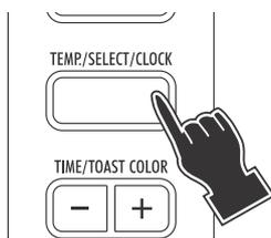
2 If necessary, the desired temperature can be modified by pressing repeatedly the TEMP./SELECT/CLOCK button (7). The available temperatures are: 200 - 250 - 275 - 300 - 325 - 350 - 375 - 400 - 425 - 450°F. The display will show the chosen temperature.
