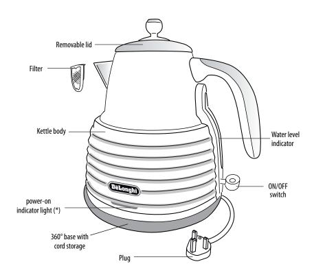
(\*) in some models the indicator light is visible only when the ON/OFF switch is depressed.
