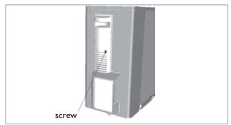
Press the handle downwards and remove the panel protecting the terminals in order to carry out the electrical connection.
