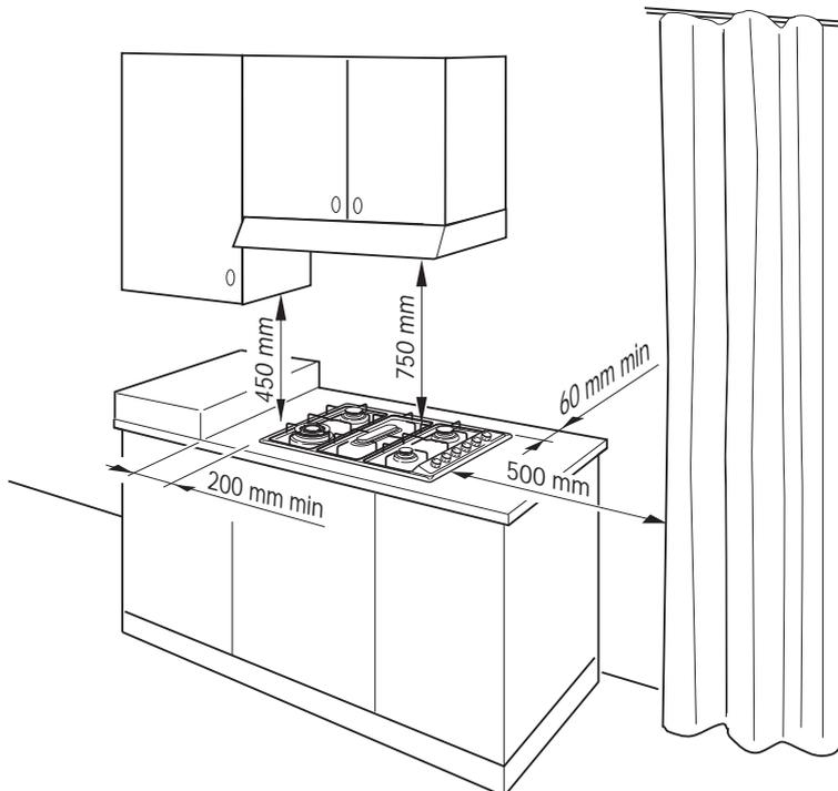
The installation shall comply with the dimensions in Figures 1 and 2, bearing in mind that:
