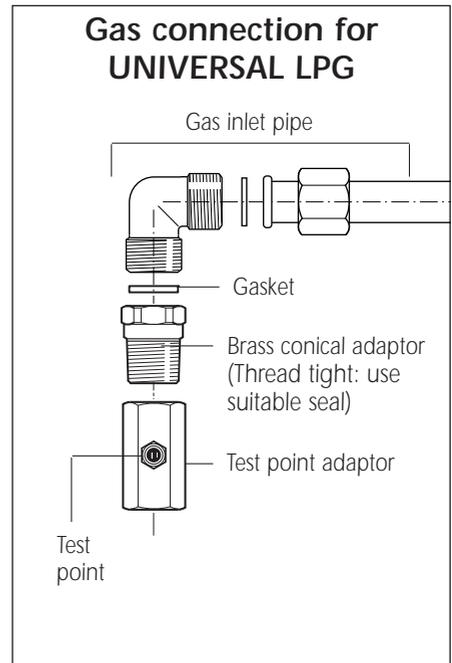
1. After connecting the gas supply, check the piping and connections for leaks using a soap and water solution. The presence of bubbles indicates a leak, tighten or replace connections as appropriate.
