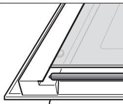
It is normal the opened gap between the top edge of the inner glass and the sealed gasket. This allows the cooling air circulation
