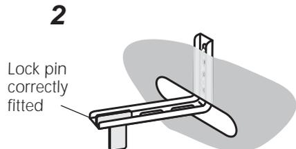
Figure 5c Fitting the lock pin through the bracket
