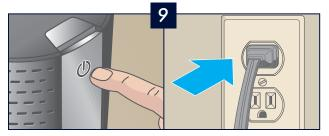
To reset Change Filter notification, press in the ON/OFF button while at the same time plugging the unit into an outlet.
