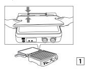
Each plate can be inserted in either the upper or lower housing (see figure 2).
