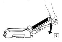
Lifting the handgrip slightly before press the hinge release button lightens pressure on the hinge and facilitates the operation.
