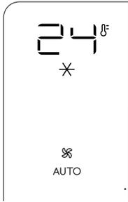
This is ideal for hot and humid weather when the room needs to be both cooled and dehumidified.
