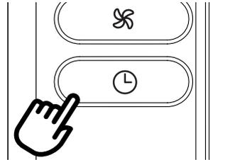
The timer allows the delayed start up or shut down of the appliance. This function will prevent wasting electricity by optimising the operating periods.
