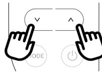
The temperature can be displayed in °C or °F. To change the temperature unit of measure touch both the increase ^ (C4) or decrease v (C3) keys for about 10 sec.
