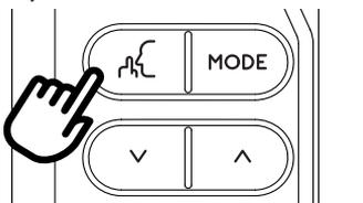
By activating this function, the operating noise is further reduced. To activate it, press (D2) button on the remote control. The display shows the relative symbol (C12).
