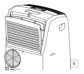
The silver ion filter not just retains dust particles, but also has an efficient antibacterial action. It also greatly reduces concentrations of irritants such as pollen and spores.
