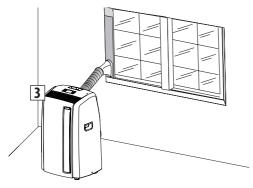
If you have a casement window (figure 4) follow steps 2 & 3 and place the window outlet **B3** outside the window to exhaust the hot air.
