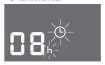
The timer can be used to delay appliance start up or shutdown. This avoids wasting electricity by not operating the appliance when it is not needed.
