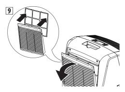
Use a vacuum cleaner to remove the dust collected on the filter. If it is very dirty, immerse in warm water and rinse a number of times. The water should never be hotter than  $104^{\circ}F$  ( $40^{\circ}C$ ). After washing the filter, allow it to dry completely before repositioning it.
