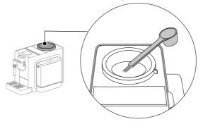
Locate the bean hopper in the socket, being sure to align the unlock position  $\square$  with the notch on the machine
