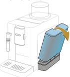
Tilt the tank away from the machine: once released, it will detach easily.
