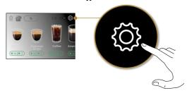
Scroll through the pages until the item "Rinse" is displayed and press "Yes" to start the procedure: after a few seconds, hot water will begin flowing to clean and heat up the internal circuit of the
