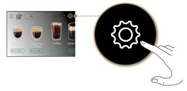
Scroll through the pages until the item "Coffee temperature" is displayed and press "Set" to change the temperature.
