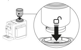
Twist the bean hopper clockwise to the point at which the lock position  $\triangle$  aligns with the notch on the machine
