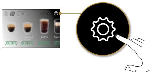
*Scroll through the pages until the item “Rinse” is displayed and press “Yes” to start the procedure: after a few seconds, hot water will begin flowing to clean and heat up the internal circuit of the machine.*
