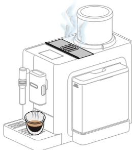
*This is water vapour that escapes from the dose of coffee utilized and is released automatically by way of the grounds container. This happens as part of normal and correct operation.*
