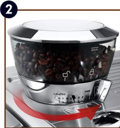
2 The ideal setting depends on your coffee bean type. The factory default is 5 but for a finer or coarser grind we invite you to check on the **coffee guide settings table**. **If you need to adjust, do it while grinding.**
