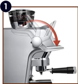
1 After grinding, pull the lever down fully (do not remove portafilter). For a perfect result, you can do it twice.
