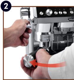
2 Keep the lever down while removing the portafilter. Once it is done, place back the lever in its original position.
