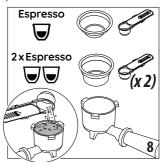
Fill the cup filter with ground coffee using the measuring spoon (A18). Make sure that you are using a fine grind, specific for espresso.
