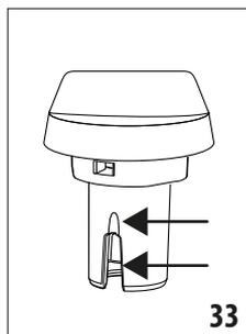
Make sure there are no milk residues on the hollow and groove under the dial (fig. 33). If necessary, scrape the groove with a toothpick;
