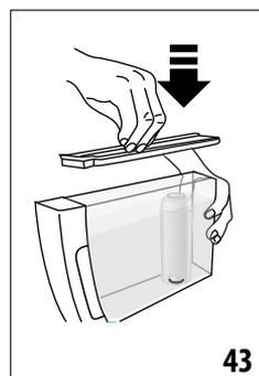
4. Remove the tank (A11) from the machine and fill with water. Insert the filter in the water tank and immerse it completely for about ten minutes, sloping it to enable the air bubbles to escape (fig. 41).
