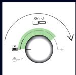
The machine is pre-set on minimum. Based on type of coffee find the right dose by gradually turning the dial within the green are
