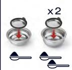
Select single or double filter. For double filter press "X2" before grinding.
