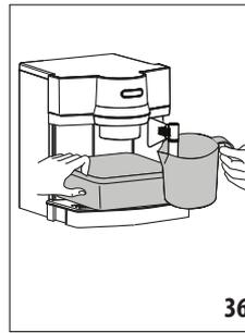
1. Empty the water tank (A8) completely and remove the water softener filter (C10) (if present). Fill the tank with the descaler solution, obtained by diluting the descaler with water following the instructions on the pack;
