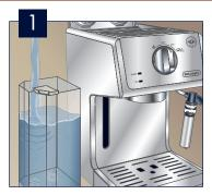
Remove tank, fill with water and replace.
