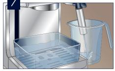
Then turn the steam dial to the 🗁 🙈 position and discharge all the water remaining in the tank from the cappuccino maker. Turn the steam dial back to and the selector dial to ON position to stop the flow.
