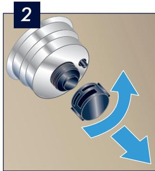
2 Unscrew cap from the steel filter cup.
