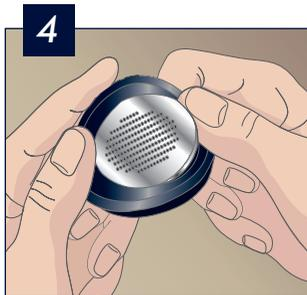
4 Remove the filter from the the gasket.
