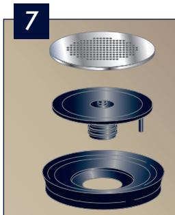
7 Replace the filter and plastic disc into the gasket. Make sure to insert the pin on the plastic disc into the hole in the gasket.
