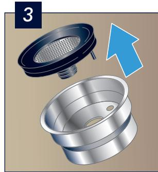
3 Remove gasket from the steel filter cup.
