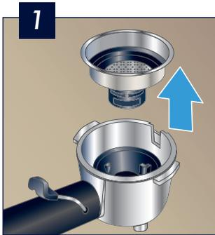
1 Remove steel filter cup from the steel filter holder.
