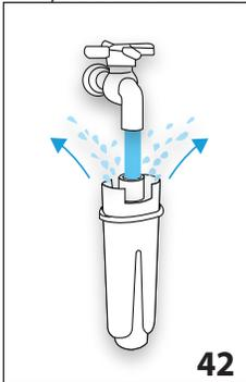
5. "RUN WATER INTO FILTER HOLE UNTIL IT COMES OUT" (fig. 42): To activate the filter, run tap water through the hole in the filter as shown in the figure until water comes out of the openings at the side for more than a minute. Press the selection arrow corresponding to "NEXT>";
