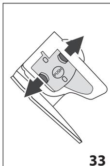
8. Once inserted, make sure the two coloured buttons have snapped out (fig. 33);
