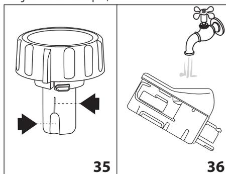
5. Rinse inside the froth adjustment dial seat with running water (fig. 36);
