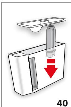
12. (If the filter is installed) "INSERT FILTER INTO ITS HOUSING" (fig. 40). Press "NEXT>" and extract the water tank. Replace the water softener filter if removed previously;
