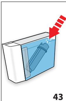
7. "IMMERSE FILTER TO EXPEL AIR BUBBLES" (fig. 43): Insert the filter in the water tank and immerse it completely for about ten seconds, sloping it and pressing it lightly to enable the air bubbles to escape. Press the selection arrow corresponding to "NEXT>";
