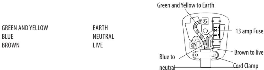
As the colours of the wires in the mains lead of this appliance may not correspond with the coloured markings identifying the terminals in your plug, proceed as follows:
