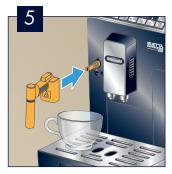
Insert water spout and place a container underneath.
