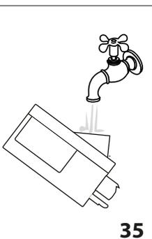
5. Rinse inside the froth adjustment dial seat with running water (fig. 35);
