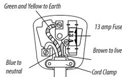
As the colours of the wires in the mains lead of this appliance may not correspond with the coloured markings identifying the terminals in your plug, proceed as follows:
