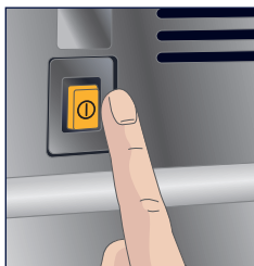
Push ON main switch, located on back of machine.
