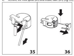
Remove the froth regulator (D1) by pulling it outwards (fig. 36); 4. Wash all the components thoroughly with hot water and mild washing-up liquid.
