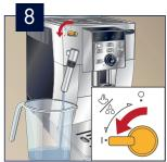
Turn dial counter-clockwise to start the prime. Water will be released by the hot water/steam spout: the machine will then switch it off automatically.
