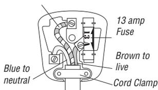
As the colours of the wires in the mains lead of this appliance may not correspond with the coloured markings identifying the terminals in your plug, proceed as follows:
