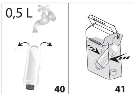
4. Extract the tank from the appliance and fill with water.
