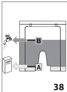
7. Pour the descaler into the tank up to level A (corresponding to a 100 ml pack) marked on the back of the tank (fig. 38), then add water (1 litre) up to level B (fig. 38) and put the water tank back.
