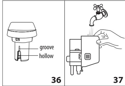
5. Rinse inside the froth adjustment dial seat with running water (fig. 37).
