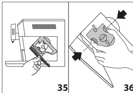
4. Press the two red release buttons inwards and at the same time pull the infuser outwards (fig. 36).
