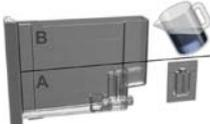
4. "ADD DESCALER, FILL WATER TANK" "INSERT WATER SPOUT" is displayed.
