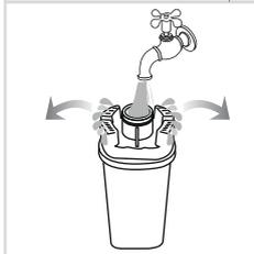
3. To activate the filter, let tap water go in the hole of the filter as shown in the figure as long as the water comes out from the side openings for over one minute.
