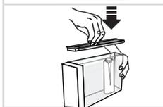
6. Insert the filter in the filter housing and press as far as it will go.
