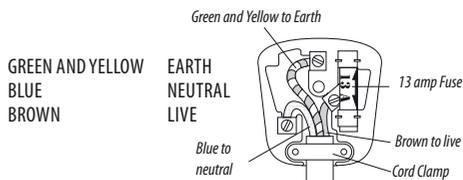
As the colours of the wires in the mains lead of this appliance may not correspond with the coloured markings identifying the terminals in your plug, proceed as follows:
