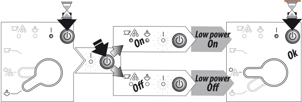
When LOW power is enabled, the device will automatically activate LOW POWER after 15 minutes and subsequently go into standby mode.
