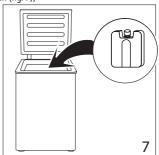
6. Put the ice box/pack vertically in the front left corner of the tank as shown in figure 8;
