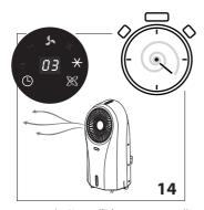
If you want to exit the "Auto off" function, repeatedly press the button (B6 or D3) until "00" is displayed: symbol flashes then disappears and "Auto Off" function is disabled.
