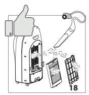
Wash thoroughly the cooling pad with water; then leave it to completely dry and reassemble the filters in its housing (fig. 19).
