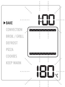
The values that can be changed, cooking time and temperature, flash. If these values are not set, the display will show 1:00 h and 180°C.
