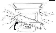
After cleaning, put the heating element back in position.
