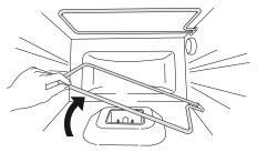
After cleaning, put the heating element back in position.
