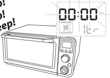
The control is now in 'waiting mode'. In this state you can add up to 10 minutes, if necessary, to complete the cooking. This state is kept for 5 minutes, after that the control will turn off the oven automatically.
