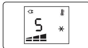
In this operation mode the working power can not be set. The appliance will automatically set to Max power level. If you turn the dial clockwise, you will restore the same power setting as before being switched to anti-frost.
