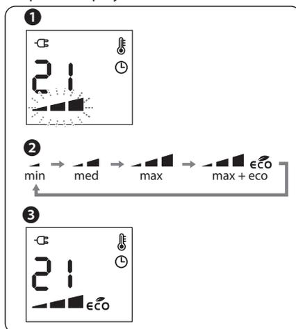
**i Please note:** If a procedure to modify or monitor the unit settings is interrupted and no button is pressed for two minutes, the settings shown on the display will not be maintained and the appliance will go back to the settings previously displayed.
