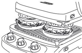
The grease from the food is drained and collected by the grooves on the plate and the hole at the corner.
