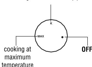
**D2 - BOTTOM PLATE THERMOSTATE**
