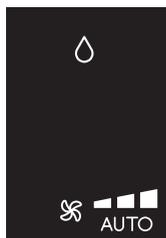
This is ideal for reducing humidity in the room (spring and autumn, damp rooms, rainy periods, etc). For this type of use, the appliance must be set up as for air conditioning mode. That is, the air exhaust hose (B2) must be fitted to the appliance to allow the humidity to be discharged outside.
