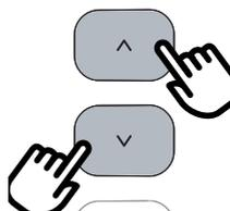
The temperature can be displayed in °C or °F. To change the temperature unit of measure touch simultaneously for ten seconds the increase ^ (C3) and decrease v (C4) key.
