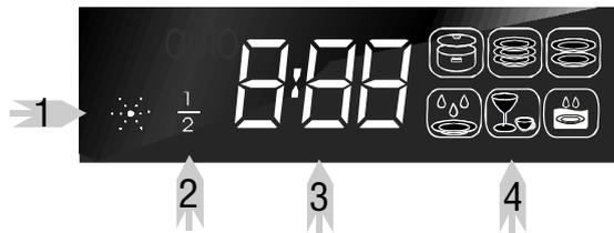
Display Window: Program remaining time, delay time, temperature of water, fault codes and etc.
