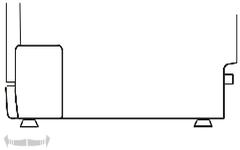
Once the appliance is positioned, adjust the feet (screwing them in or out) to adjust the height of the dishwasher, making it level. In any case, the appliance should not be inclined more than 2°.
