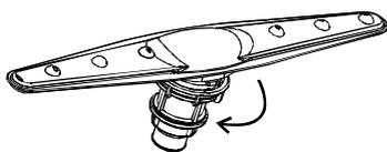
It is necessary to clean the spray arms regularly, for hard water chemicals will clog the spray arm jets and bearings. To remove the spray arm, screw off the nut clockwise to take out the washer on top of the spray arm and remove the arm. Wash the arms in soapy and warm water and use a soft brush to clean the jets. Replace them after rinsing them thoroughly.
