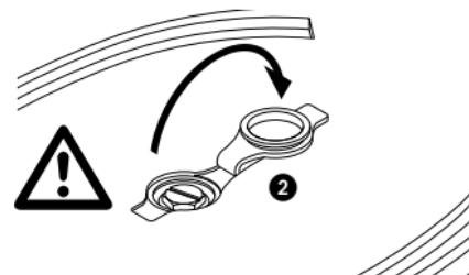
Unscrew the boiler cap using a coin and empty out any water. Add one cup of tap or filtered water and shake the appliance then empty out all the water. Repeat this operation until the water from the boiler comes out clear and clean.
