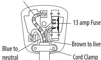
As the colours of the wires in the mains lead of this appliance may not correspond with the coloured markings identifying the terminals in your plug, proceed as follows:
