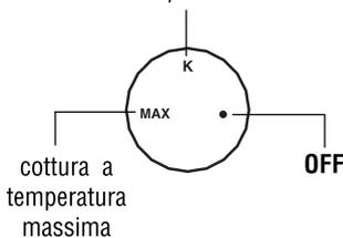
**D2 - TERMOSTATO PIASTRA INFERIORE**
