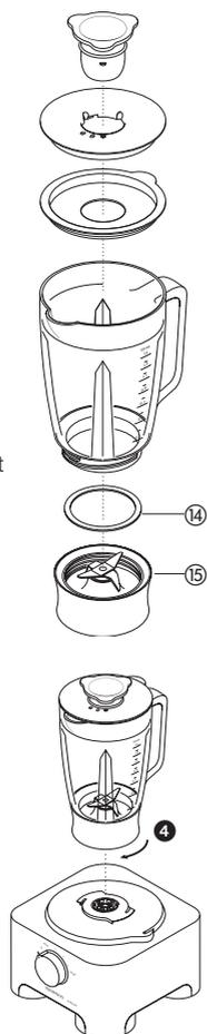
**Note: The mill base is not interchangeable with the FP920/FP930 glass liquidiser jug. The processor will not operate if the wrong base is fitted. Refer to graphics on blade unit bases.**
