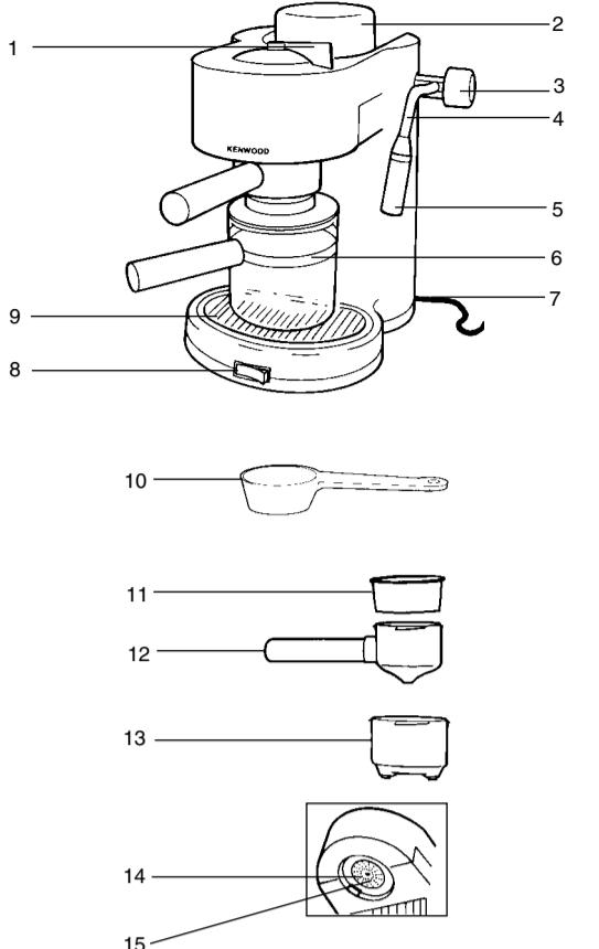
When in use the reservoir is under pressure. Before removing the reservoir cap (fig 3) or removing the filter holder always ensure that the pressure has been equalised by opening the steam control knob.
